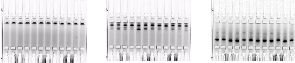
Figure 4: DNA migration through a gel cassette illustrating synchronised arrival at the extraction wells.
